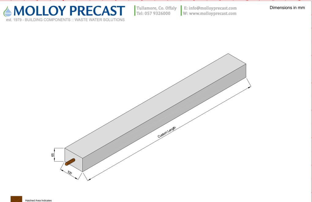
Hatched Area Indicates Pre-stressed High-Tensile Steel
